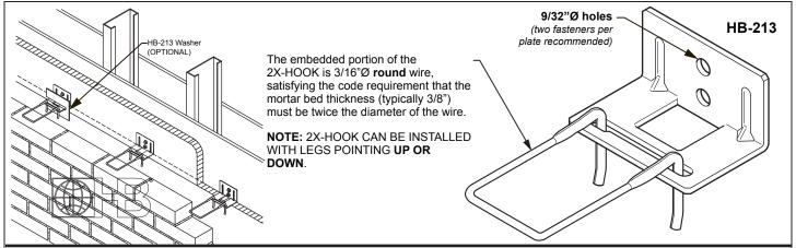
Hohmann & Barnard's 2X-HOOK has been tested and designed to withstand over 200-lbf, in tension or compression, at maximum allowed offset (TMS 402/602-16 12.2.2.5.5.4) of 11/4" (disengagement of the pintle from the veneer anchor). These results exceed BIA recommendations and the capabilities of standard "round wire" hooks/pintles by over 100%, while maintaining the ASTM A1064/1064M wire specification.
